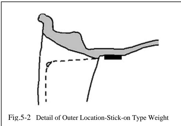
Fig.5-2 Detail of Outer Location-Stick-on Type Weight
